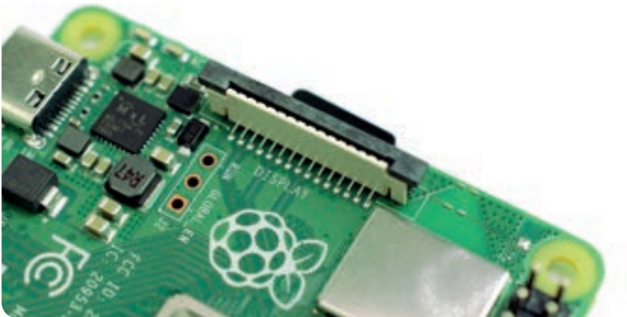
▲ Figure 1-12: Raspberry Pi's display connector (DSI)
