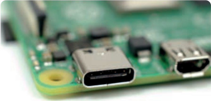
▲ Figure 1-11: Raspberry Pi's USB Type-C power port
