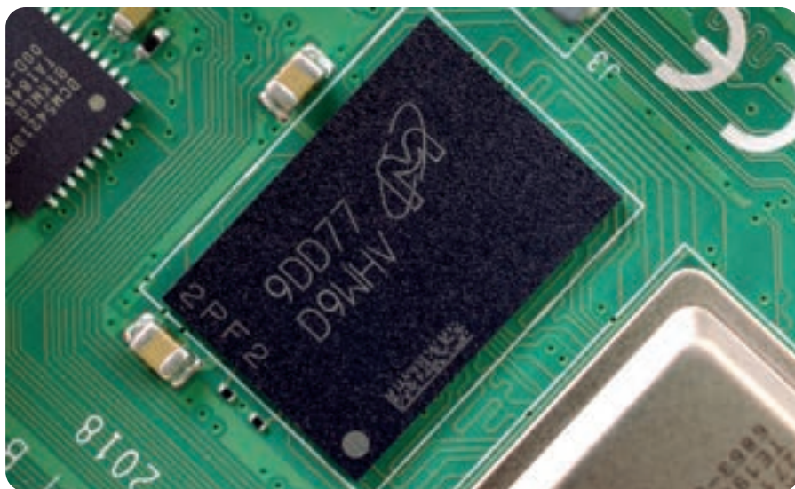
▲ Figure 1-3: Raspberry Pi's random access memory (RAM)
