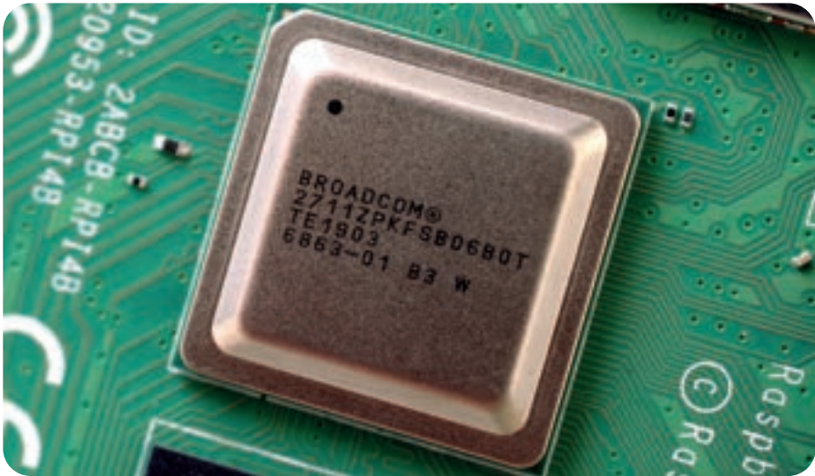
▲ Figure 1-2: Raspberry Pi's system-on-chip (SoC)
