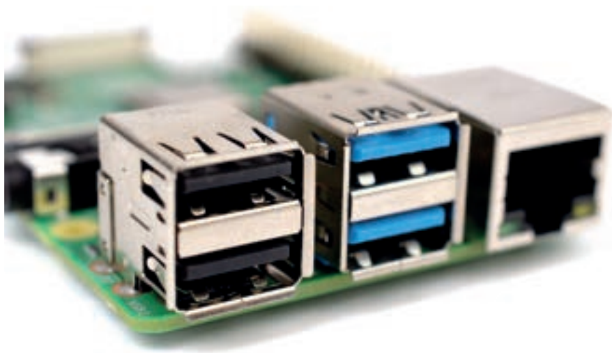
▲ Figure 1-6: Raspberry Pi's USB ports
