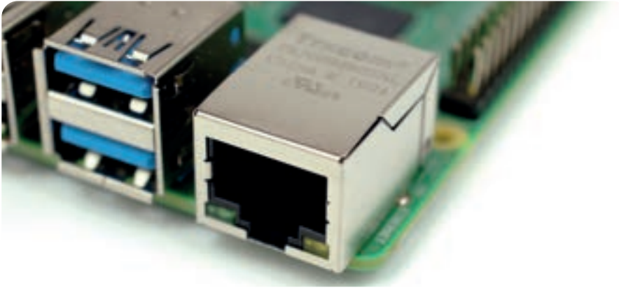
▲ Figure 1-7: Raspberry Pi's Ethernet port
