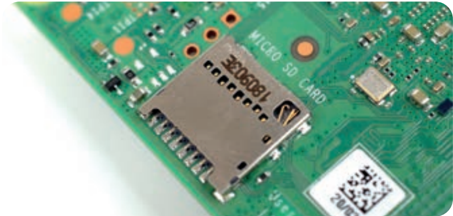
▲ Figure 1-15: Raspberry Pi's microSD card connector
